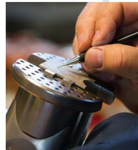
Hardy sketches a drawing on silver mounted on his engraver's ball, ready for bright-cut engraving. "If you can't draw it, you can't effectively cut it," he says.
